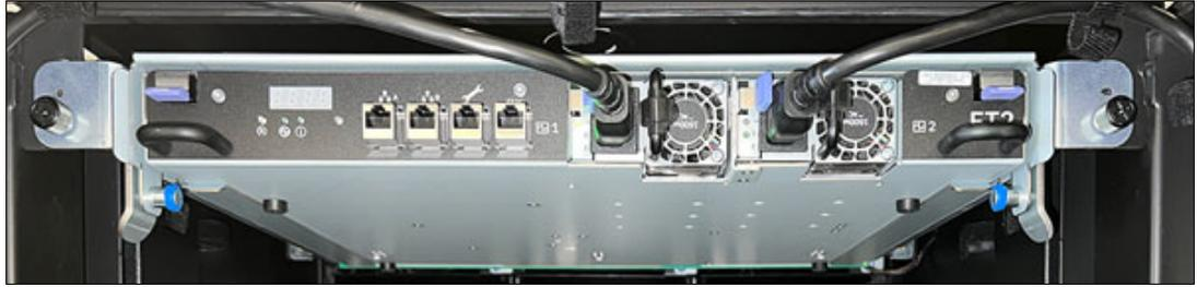
Figure 1-4 IBM Diamondback electronics tray close up
